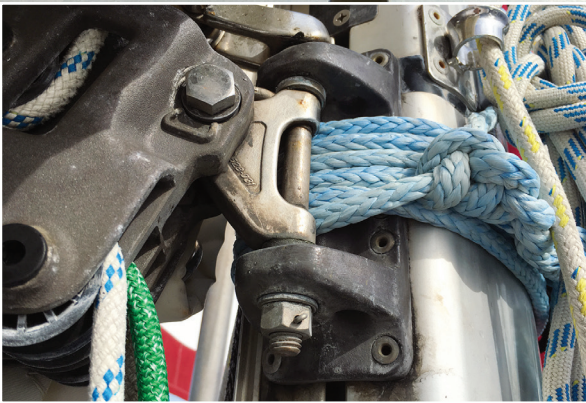
LEFT: The gooseneck mast fitting lashed to the mast to prevent it following the kicker strut
